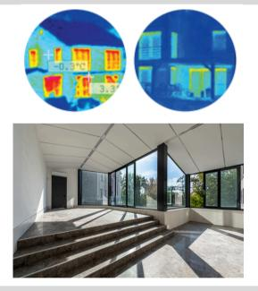
Visible Thermal Insulation Standard windows compared to insulating glass windows with TPS
