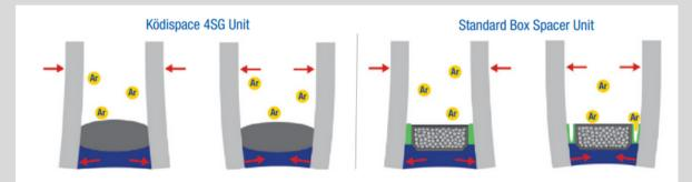
This warm edge system offers unlimited insulating glass unit (IGU) shapes and design, excellent thermal performance, maximum gas tightness and low MVTR. As a permanent flexible spacer its high elasticity and chemical bonding result in better mechanical performance during environmental changes.
